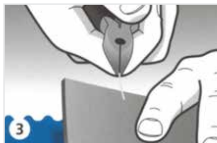
Gently pull the pin out using pliers.
